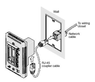
• If the end of the cable is terminated with a male connector, connect the network cable directly into the Ethernet uplink port.
